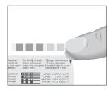
► You will then be able to read the degree of water hardness from the discolouration of the Aquadur® test strip and the description on the packaging.
